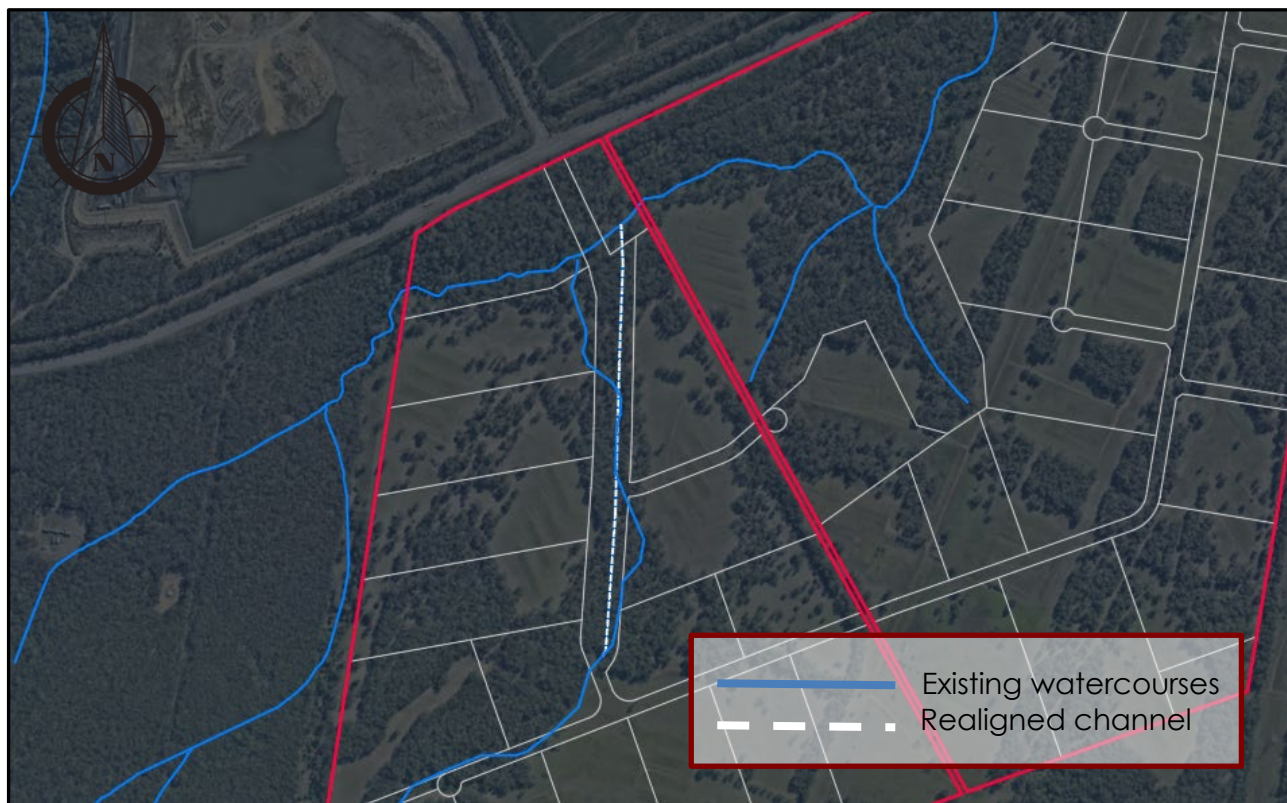
Figure 13 – Intended watercourse realignment.
